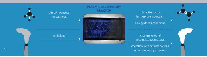
1 Illustration of possible conversion routes by gas activation with nonthermal plasma – exemplified by a plasma laboratory reactor of Fraunhofer UMSICHT.
